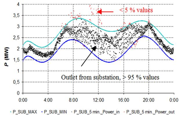
Fig. 7: Control of adjustment of power output difference thresholds.
