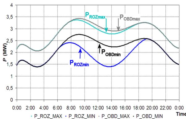
Fig. 6: Substation outlet extreme conditions.
