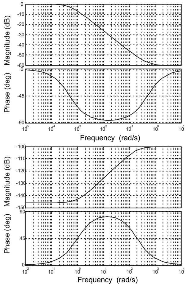
Fig. 8: Amplitude and frequency characteristics of the low-pass weighting filter  $W_e(s)$  (upper part) and high-pass weighting filter  $W_u(s)$  (lower part): mathematical model in elevation.
