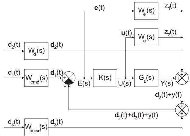
Fig. 6: Block diagram of the connection of the  $H_\infty$  robust controller, nominal system and weighting filters for the helicopter model.
