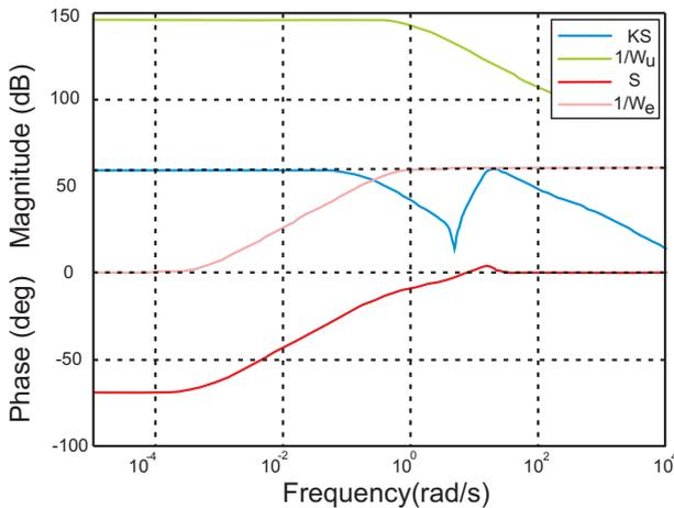
**Fig. 10:** Amplitude frequency characteristics of the sensitivity function  $S(s)$ , product of transfer functions  $K(s)S(s)$ , inverted transfer functions  $1/W_e(s)$  and  $1/W_u(s)$ : mathematical model in elevation.
