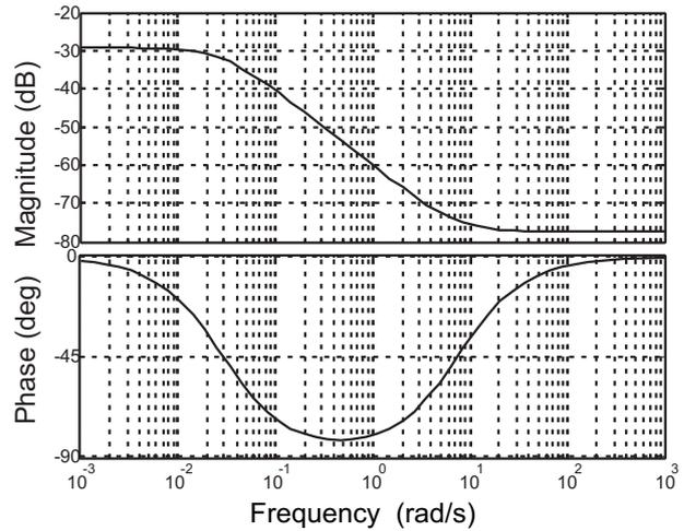
Fig. 13: Amplitude and phase frequency characteristics of low-pass filter  $W_e(s)$ , real model in elevation.
