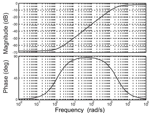
Fig. 14: Amplitude and phase frequency characteristics of high-pass weighting filter  $1/W_u(s)$ , real model in elevation.
