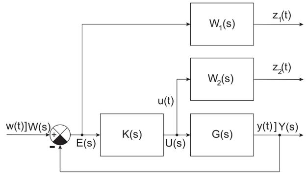
Fig. 4: Standard block diagram of the mixed sensitivity problem: controller and perturbed system containing nominal system, control error and manipulated value weighting filters.
