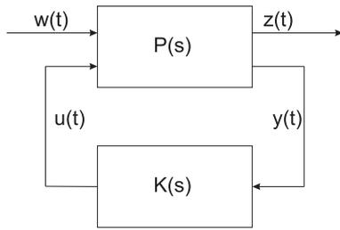
Fig. 3: Standard block diagram at the  $H_\infty$  configuration.
