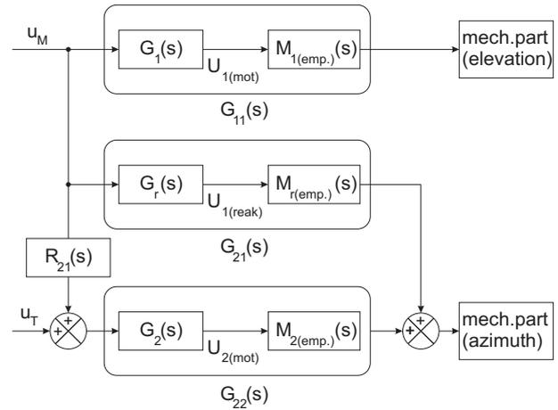
Fig. 5: Block diagram for the elimination of the elevation-azimuth coupling; the azimuth-elevation coupling is neglected.
