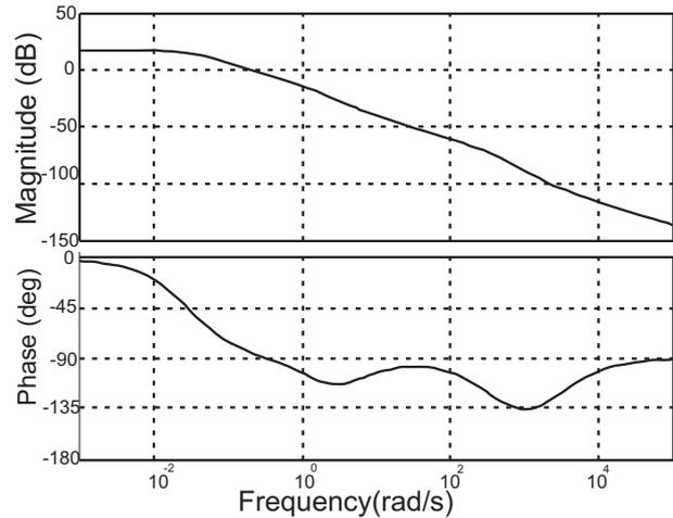
Fig. 17: Amplitude frequency characteristic and phase frequency characteristic of the  $H_\infty$  controller for real model in elevation.
