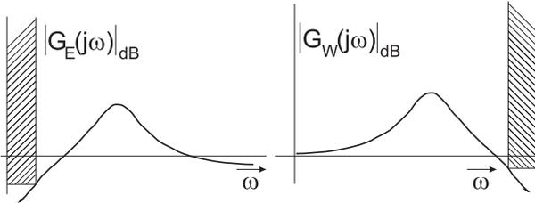
Fig. 2: Logarithmic amplitude frequency characteristics for the sensitivity function (on the left) and complementary sensitivity function (on the right).
