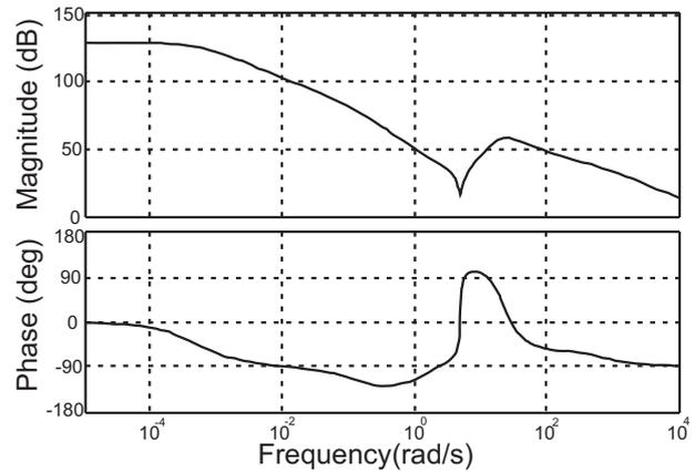
**Fig. 11:** Amplitude frequency characteristic and phase frequency characteristic of the  $H_\infty$  controller for mathematical model in elevation.
