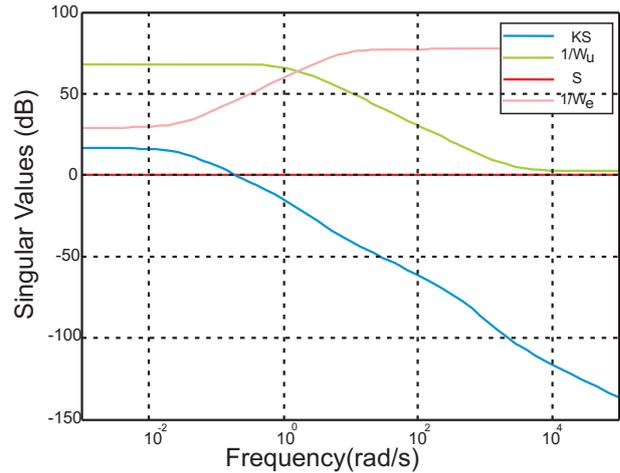
Fig. 16: Amplitude frequency characteristic of the sensitivity function  $S(s)$ , product of transfer functions  $K(s)S(s)$ , inverted transfer functions  $1/W_e(s)$  and  $1/W_u(s)$ , real model in elevation.
