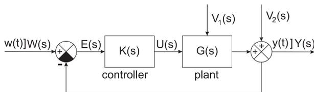
**Fig. 1:** Classical control scheme with the definition of circuit signals.
