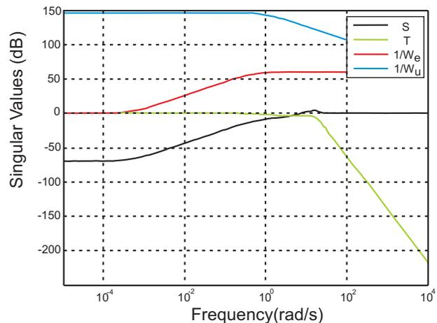
Fig. 9: Amplitude frequency characteristic of the sensitivity function  $S(s)$ , complementary sensitivity function  $T(s)$ , inverted transfer functions  $1/W_e(s)$  and  $1/W_u(s)$ : mathematical model in elevation.
