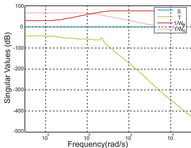
Fig. 15: Amplitude frequency characteristics of the sensitivity function  $S(s)$ , complementary sensitivity function  $T(s)$ , inverted transfer functions  $1/W_e(s)$  and  $1/W_u(s)$ , real Mmodel in elevation.
