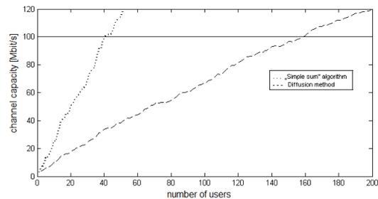
Fig. 9: The simulation results for „Simple sum“ algorithm and diffusion method.
