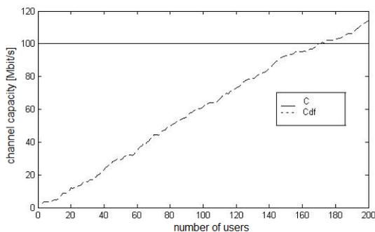
Fig. 4: The resultant statistical effective bandwidth  $C_{df}$ .
