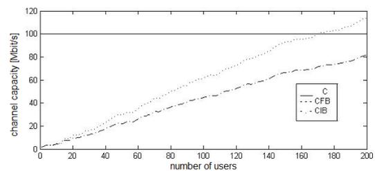
Fig. 5: Statical bandwidth with finite  $C_{FB}$  and infinite  $C_{IB}$  buffer size.
