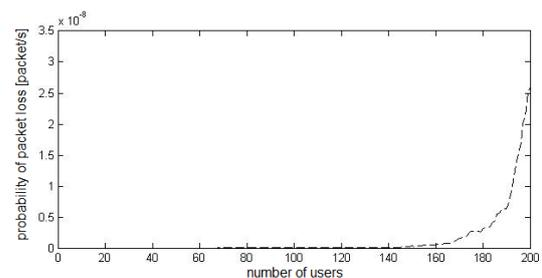
Fig. 6:  $P_{FB}$  - The probability of packet loss with a finite buffer size.
