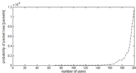
Fig. 7:  $P_{IB}$  - The probability of packet loss with an infinite buffer size.
