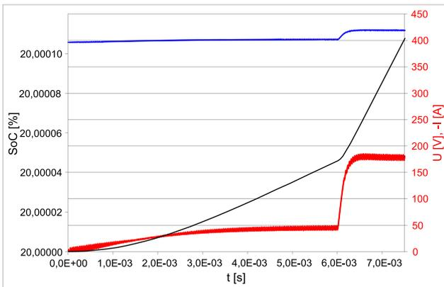
Fig. 5: Waveforms of variables in the battery of charged EV with charging current 45 A in time interval (0–6) ms and 180 A after 6 ms.
