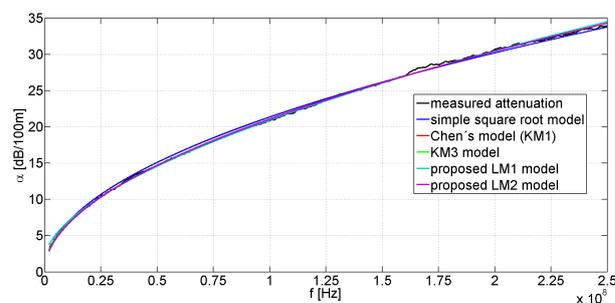
Fig. 1: Measured and modeled attenuation constants for UTP cat. 5.
