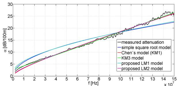
Fig. 11: Results of attenuation constant for TCEPKPFLE cable.
