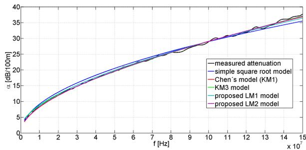
Fig. 9: Results of attenuation constant for SYKFY cable.
