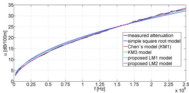
Fig. 3: Measured and modeled attenuation constants for UTP cat. 6.
