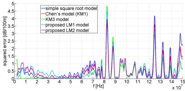
Fig. 8: SXKFY cable squared error characteristics.
