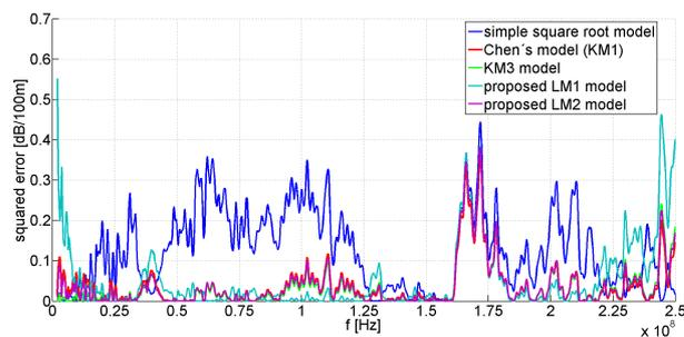
Fig. 2: Squared error characteristic for each model for UTP cat. 5.
