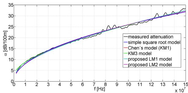
Fig. 7: Results of attenuation constant for SXKFY cable.
