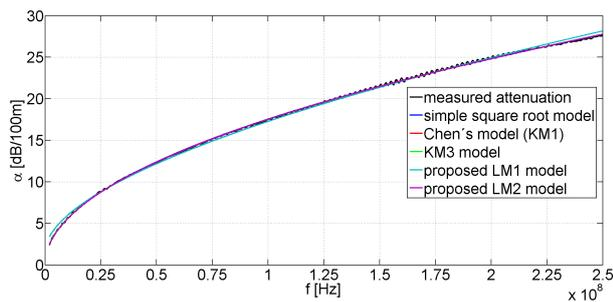
Fig. 5: Measured and modeled attenuation constants for STP cat. 7.
