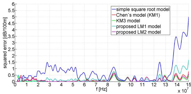
Fig. 10: SYKFY cable squared error characteristics.
