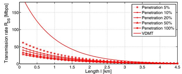
**Fig. 2:** Model of the VDSL2 length transmission rate dependence for downstream.
