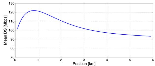
Fig. 3: The total VDSL2 downstream transmission rate on location of external DSLAM dependence.
