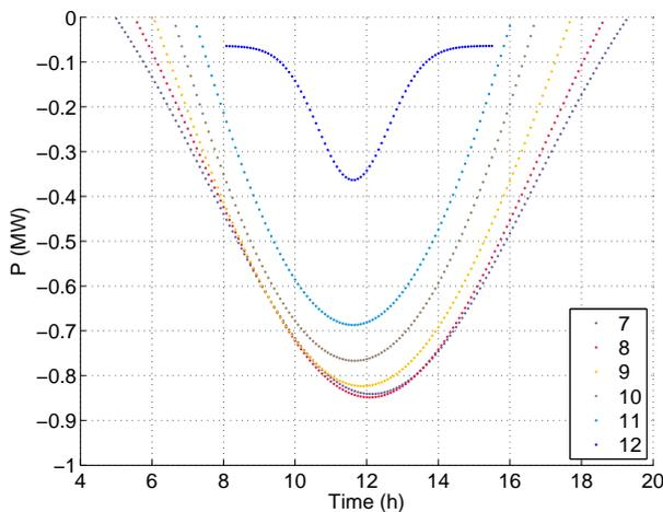
Fig. 2: Regression curves of maximum extreme outputs for individual months (July to December).
