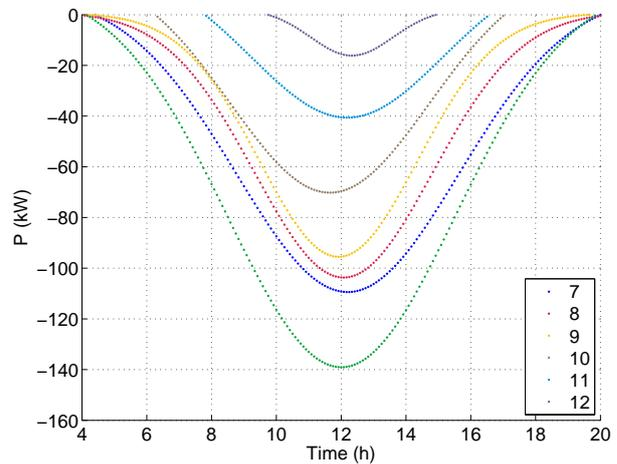
**Fig. 5:** Regression curves of minimum extreme outputs for individual months (July to December).
