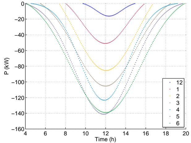
**Fig. 4:** Regression curves of minimum extreme outputs for individual months (December to June).
