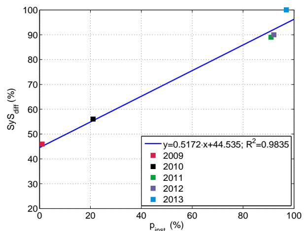
Fig. 7: Correlation analysis of the difference in system deviation and installed capacity of PvP.
