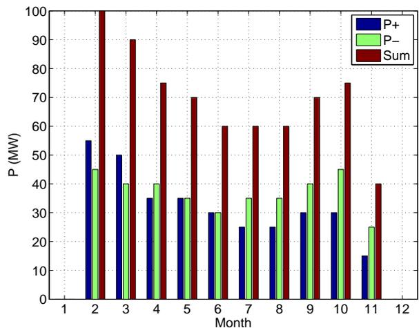
Fig. 10: Monthly values of positive and negative values of the regulatory output.
