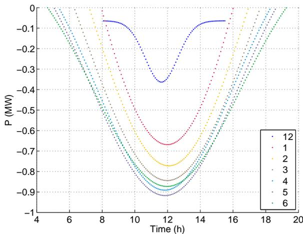
Fig. 1: Regression curves of maximum extreme outputs for individual months (December to June).
