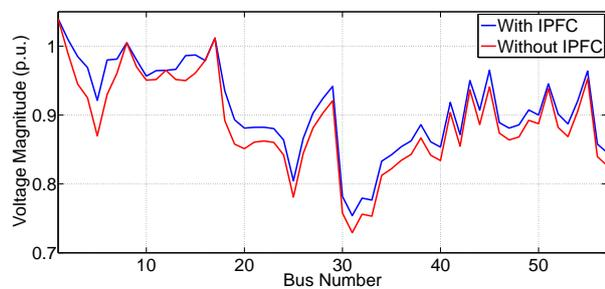
Fig. 10: Voltage profile without and with IPFC.
