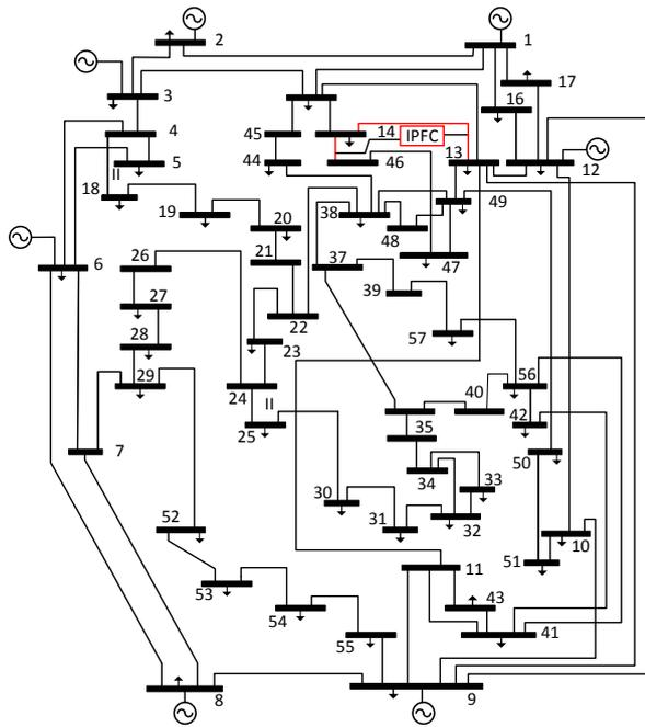
Fig. 8: IEEE-57 Bus test system with IPFC installed at line connected between buses 14-46 and 13-14.
