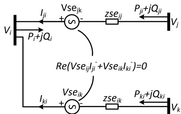
Fig. 2: Equivalent circuit of IPFC.
