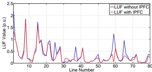
Fig. 9: Comparison of LUF values with and without IPFC with normal load.
