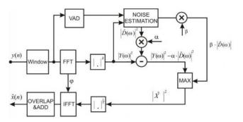
Fig. 3: Block diagram of modified spectral subtraction.
