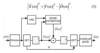
Fig. 1: General representation of spectral subtraction.
