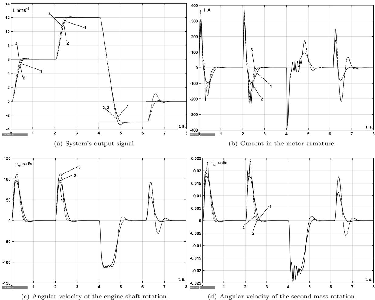
**Fig. 4:** Results of the studied system simulation 1 - with traditional controller; 2 - system with subsystem that utilizes a standardBesselform 3 - system with unstable subsystem.
