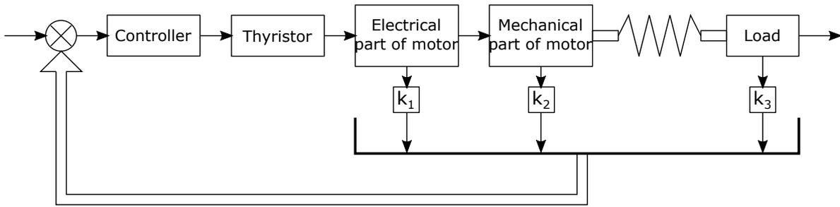
Fig. 2: Structural scheme of the two-mass system with the engine's electric component.
