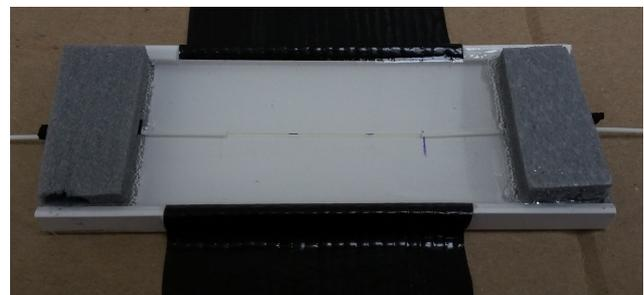
Fig. 5: Realization of encapsulation of FBG.
