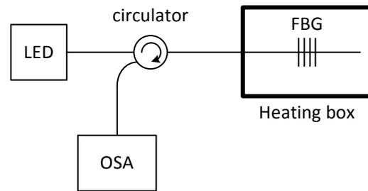
Fig. 3: Scheme of measurement with heating box.
