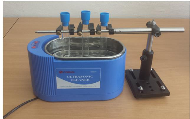
Fig. 4: Used ultrasonic bath for preparing Sylgard 184 mixture in the ratio 10:1.
