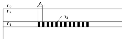
Fig. 2: Structure of fiber Bragg Gratings.
