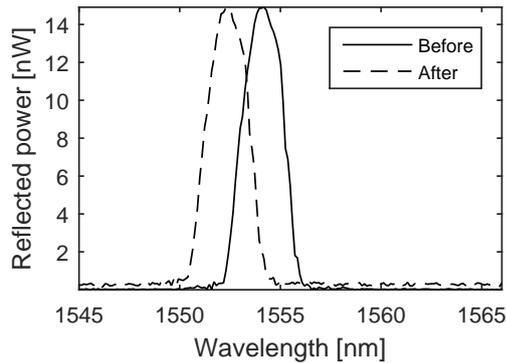
**Fig. 7:** The spectral characteristic of FBG before and after curing.
