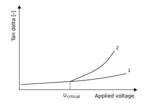
Fig. 2: Dissipation factor versus applied voltage.
