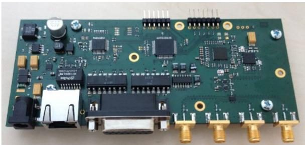
Fig. 4: AutoEPCIS UHF RFID reader – the view from above.
