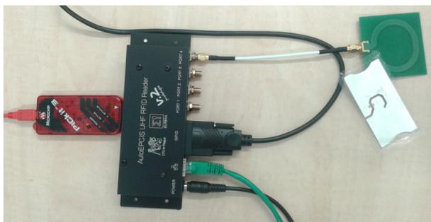
Fig. 6: Test bench – details of the RFID reader connection.
