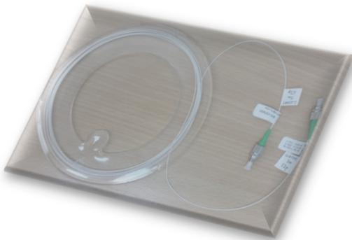
Fig. 2: Our noninvasive fiber-optic measurement probe.
