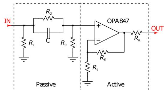
Fig. 2: Circuit diagram of active pre-equalizer with OPA847.
