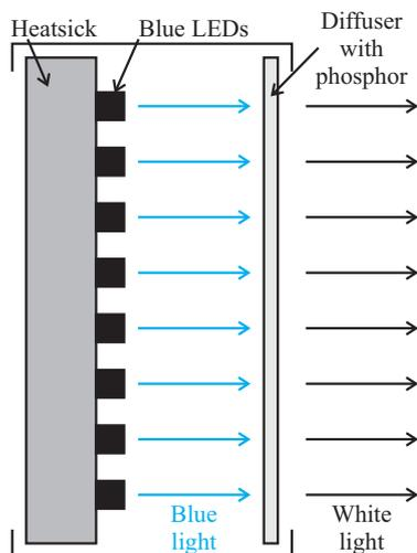
Fig. 1: Concept of Philips FORTIMO LED DLM 3000.
