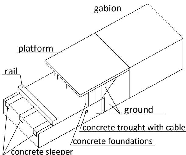
Fig. 1: Geometric layout of the model.
