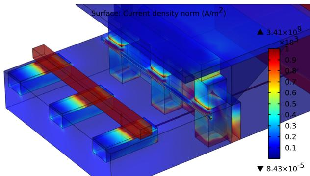
Fig. 5: Distribution of current density, concrete foundations in detail.
