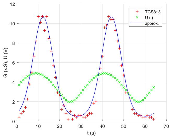
Fig. 1: The electrical conductivity  $G(t)$  of the sensor TGS 813 at frequency  $f = 0.0312$  Hz in the clean air.  $U(t)$  is the heating voltage.
