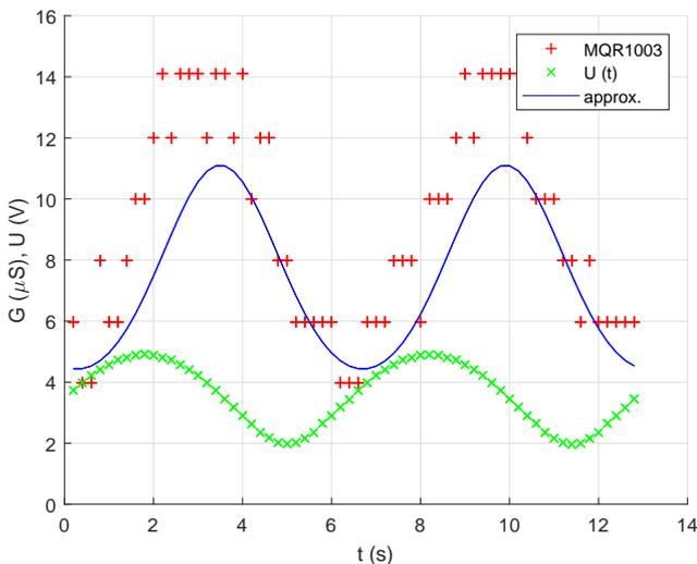
**Fig. 6:** The electrical conductivity  $G(t)$  of the sensor MQR 1003 for ethanol of the concentration  $x = 100$  ppm at frequency  $f = 0.156$  Hz of the heating voltage.  $U(t)$  is the heating voltage.
