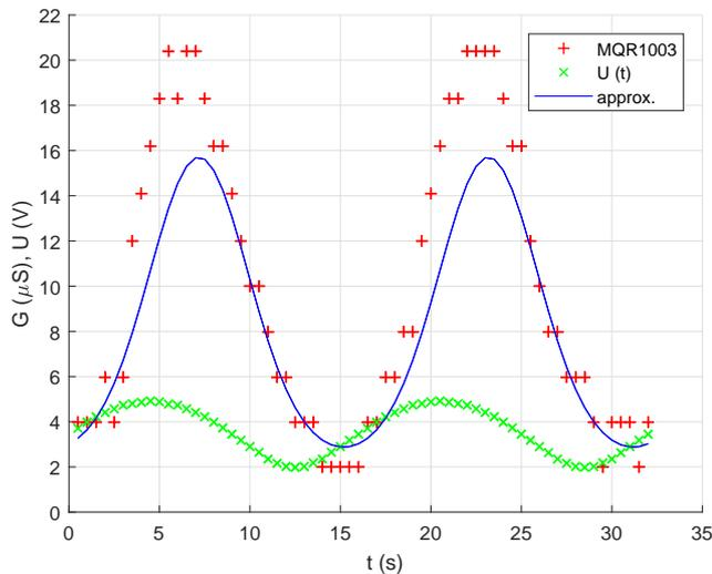
**Fig. 5:** The electrical conductivity  $G(t)$  of the sensor MQR 1003 for ethanol of the concentration  $x = 100$  ppm at frequency  $f = 0.0625$  Hz of the heating voltage.  $U(t)$  is the heating voltage.
