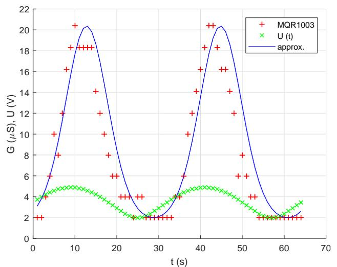
**Fig. 4:** The electrical conductivity  $G(t)$  of the sensor MQR 1003 for ethanol of the concentration  $x = 100$  ppm at frequency  $f = 0.0312$  Hz of the heating voltage.  $U(t)$  is the heating voltage.
