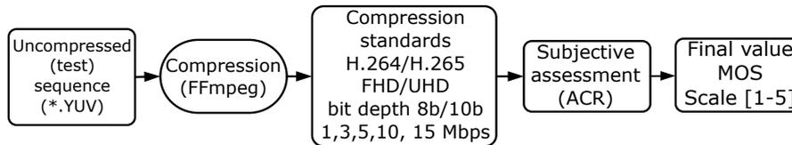
**Fig. 2:** Scheme of measurement process.
