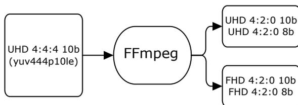
**Fig. 4:** Preprocessing of test sequences.**Tab. 3:** Command line settings of the FFmpeg tool.
