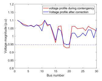
Fig. 9: Voltage profile for normal and contingency conditions.
