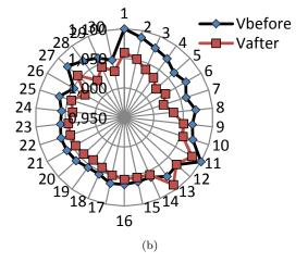
Fig. 6: a) Bus voltage magnitude case 1.2, b) Comparison of voltage profile of IEEE30 bus case 1.1 & case 1.2.
