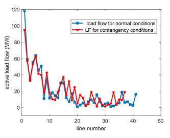
Fig. 8: Load flow profile for normal and contingency conditions.
