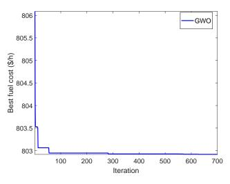
Fig. 4: Convergence characteristic of IEEE30 bus system case 1.2.
