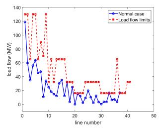
Fig. 5: Transmission Load flows obtained by GWO.
