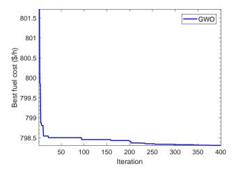
Fig. 3: Convergence characteristic of IEEE30 bus system case 1.1.
