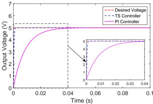
Fig. 4: Comparison between PI and T-S fuzzy controllers.
