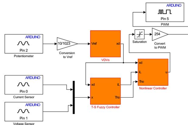
Fig. 7: Simulink model using Matlab support package.
