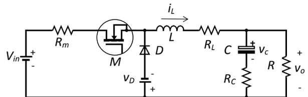
Fig. 1: Equivalent circuit of DC-DC buck converter.
