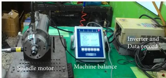
Fig. 9: Machine quality measurements.
