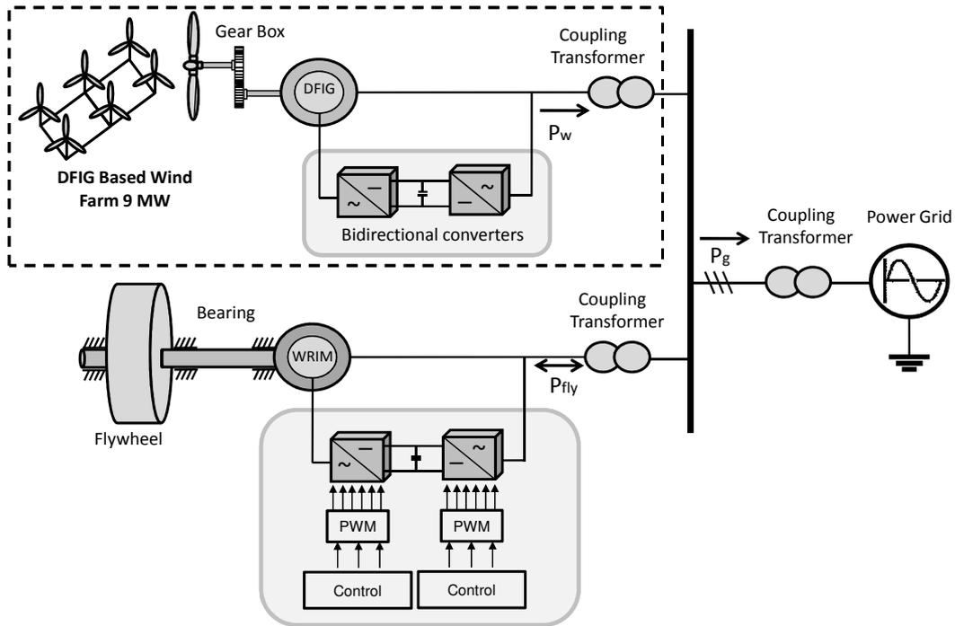
Fig. 1: WRIM driven flywheel energy storage system for wind power smoothing.
