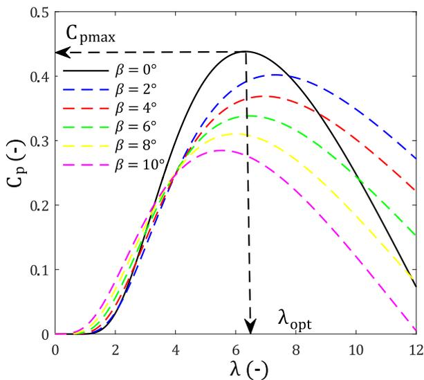
Fig. 2: Efficiency coefficient characteristic for the wind turbine.
