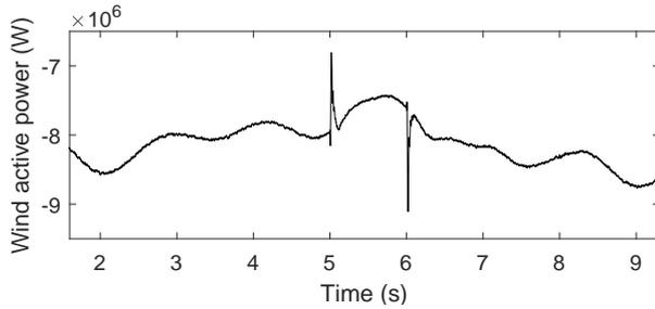
Fig. 10: Wind farm active power with voltage dip.
