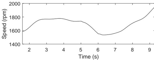
Fig. 11: WRIM rotor speed with voltage dip.
