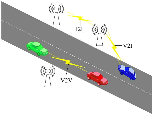
Fig. 1: Types of communication in VANET.
