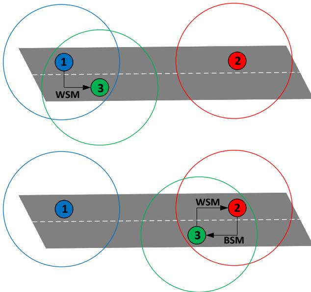
Fig. 2: Receiving information via vehicle riding in the opposite direction.
