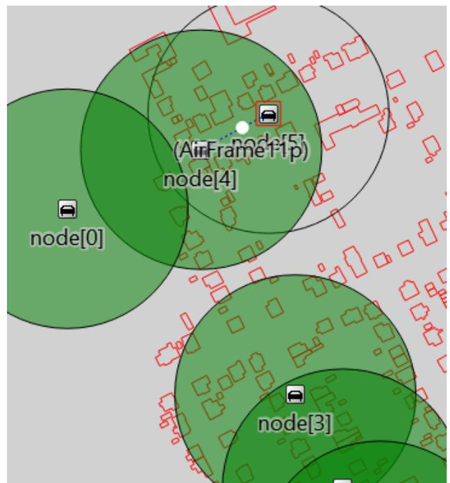
Fig. 9: Sending WSM by vehicle in the opposite traffic lane.
