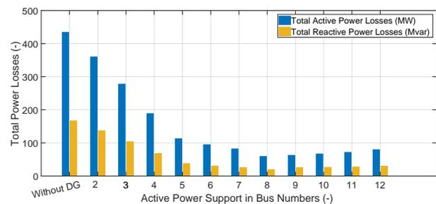
**Fig. 6:** System losses profile of the modified 12-bus with corresponding optimum DG size at each bus.
