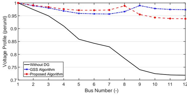
Fig. 7: Effect of DG on Voltage profile of the modified 12-bus system.
