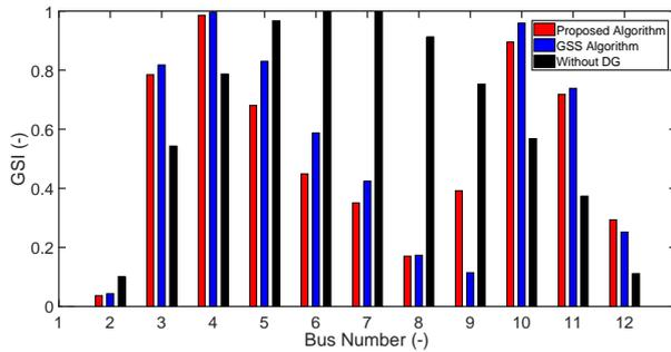
Fig. 8: Schematic GSI value for each node in a modified 12-bus system in three cases.
