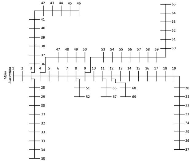
Fig. 9: Schematic diagram of 69-bus radial distribution.
