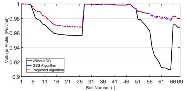
Fig. 10: Effect of DG on voltage profile of 69-bus test system.
