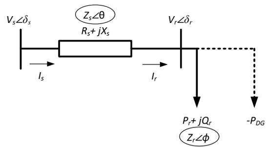
Fig. 1: Single-line diagram of a reduced system.
