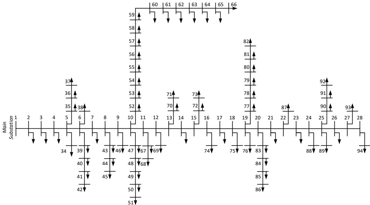
Fig. 12: Schematic diagram of 94-bus radial distribution system.
