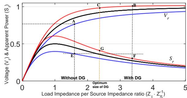
Fig. 3: Voltage and apparent power versus the load to the source impedance ratio.
