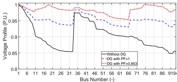
Fig. 13: Effect of DG on voltage profile of 94-bus test system.
