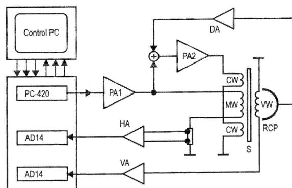
Fig. 1. Block diagram of the SST tester.
