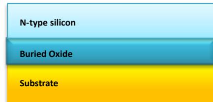
(a) n-type doped top layer of SOI wafer.
