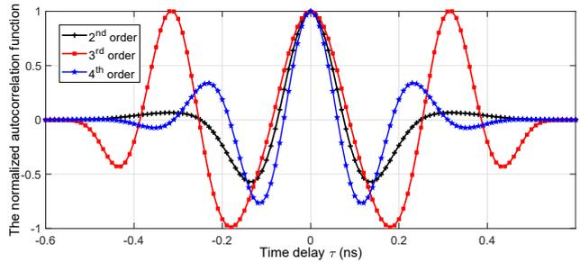
**Fig. 3:** The auto-correlation function of the Gaussian pulses as a function of time.
