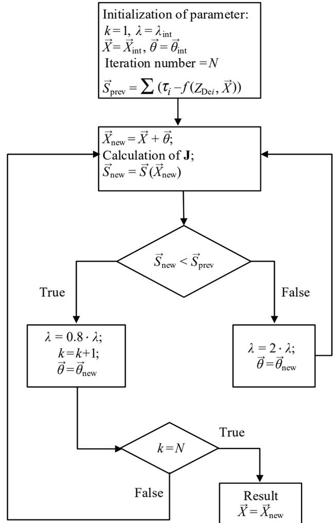
**Fig. 7:** The flowchart of CFST.
