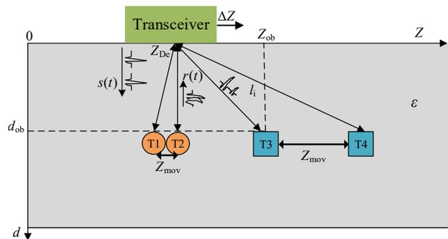
Fig. 1: The model of a UWB penetrating system.
