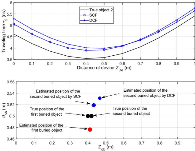
**Fig. 10:** Two adjacent buried objects: the traveling time change according to the device's translation (top) and the estimated position of the object by the CFST (bottom).
