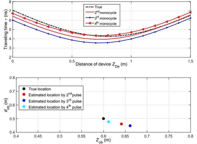
**Fig. 9:** The traveling time change according to the position of device (top) and the estimated positions of the single buried object (bottom).
