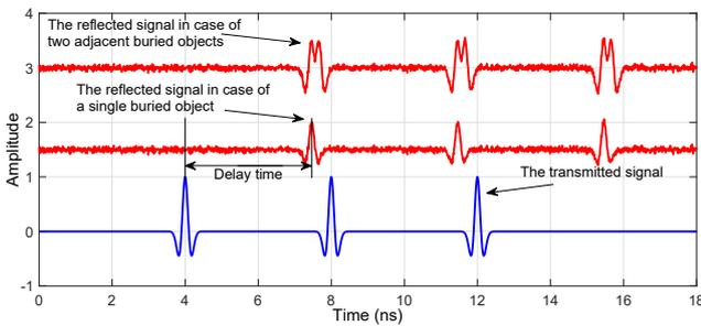
**Fig. 2:** The transmitted and reflected signals with added noise.
