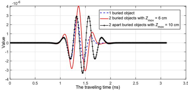
**Fig. 5:** The correlation function shapes with different distances between buried objects.
