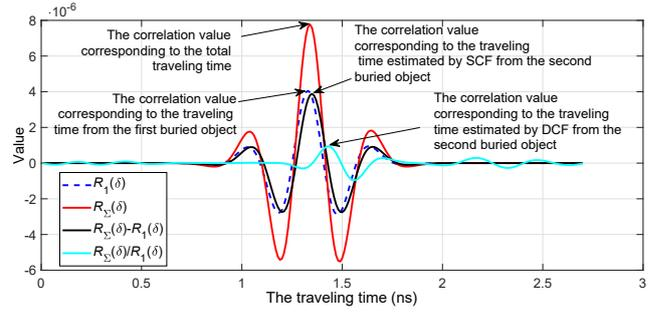
**Fig. 6:** The correlation function shapes of the reflected signals of conventional and CFST methods when there are two adjacent buried objects (the first object at  $(Z_{ob}, d_{ob}) = (0.3 \text{ m}, 0.2 \text{ m})$ ;  $Z_{mov1} = 4 \text{ cm}$ ; the transceiver is in  $Z_{Dei} = 0.3 \text{ m}$ ).
