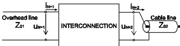
Fig. 5: Scheme of transmission overhead-cable line and interconnecting two-port
