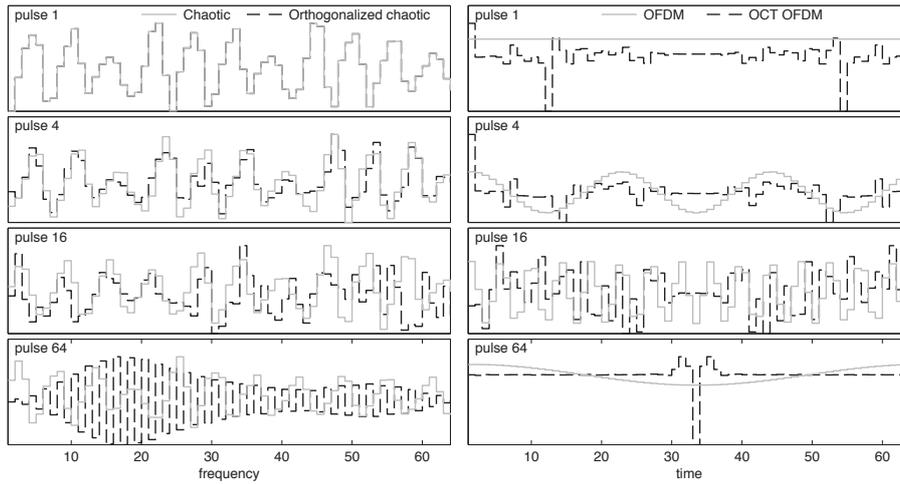
**Fig. 5:** Pulse shapes, obtained by 1/10 decimation and 64 sample grouping of composite signal from Chua’s circuit. Pulses on the right plot are obtained by applying IDFT to the OCT basis functions shown on the left plot.
