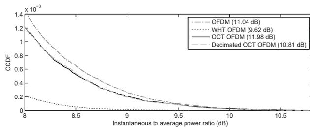
Fig. 9: CCDF tails of the baseband signals in the communication channel.
