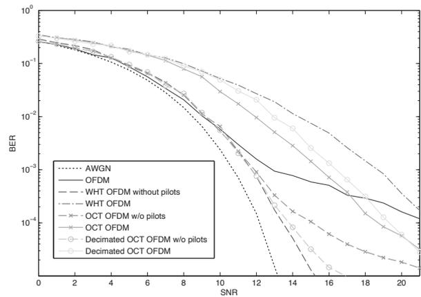
Fig. 7: Performance of the MC communication systems with different modulation schemes.
