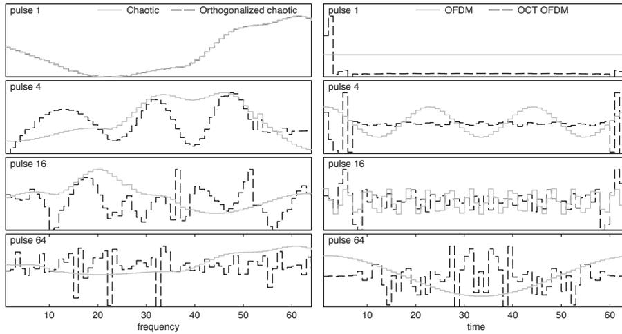
**Fig. 4:** Pulse shapes, obtained by 64 sample grouping of composite signal from Chua’s circuit. Pulses on the right plot are obtained by applying IDFT to the OCT basis functions shown on the left plot.
