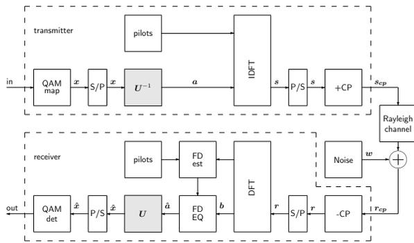
Fig. 6: Linearly precoded OFDM system model without pilot signals precoding.
