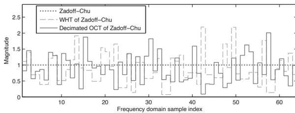
Fig. 8: Magnitude of frequency domain training signals.
