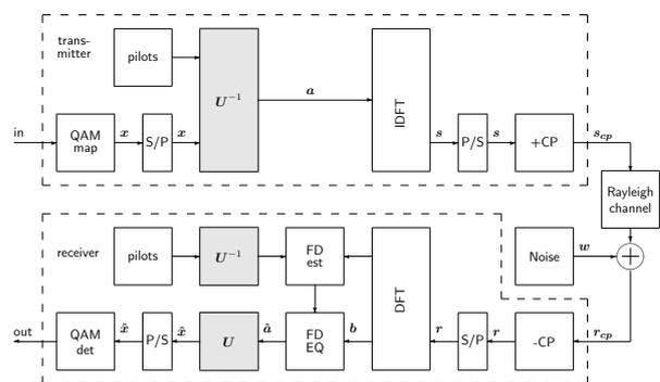
Fig. 2: Linearly precoded OFDM System Model with pilot signal precoding.
