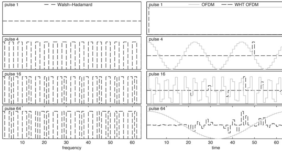
**Fig. 3:** Pulse shapes of 64 sample WHT. Pulses on the right plot are obtained by applying IDFT to the WHT basis functions, shown on the left plot.
