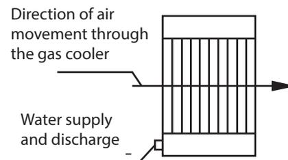
**Fig. 4:** Gas cooler with one-way movement of gas.
