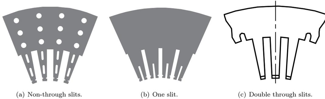
Fig. 8: Segments of the stator core with slits in the teeth.
