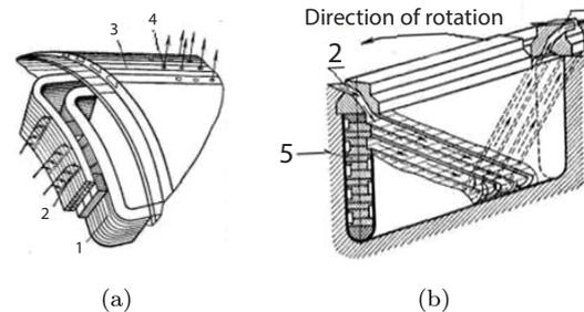
**Fig. 3:** Schemes of hydrogen supply to the conductors of the rotor winding.
