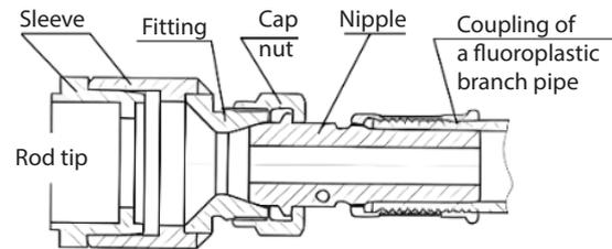
**Fig. 2:** Connection of the "cone-sphere" type for the heads of the rods of the stator winding and the tips of the fluoroplastic hoses.
