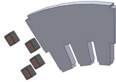
**Fig. 6:** 3D-model of the connecting elements (segment of the stator core of the turbogenerator TGV-200-2 and the winding), which was used in the simulation.
