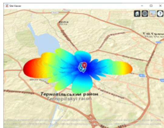
**Fig. 8:** Antenna beam scanning by applying a taper for an angle of 0 degrees in 3-dimensional coordinates.
