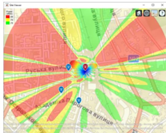
Fig. 12: Antenna beam scanning by applying a taper for an angle of +30 degrees (projection onto the terrain surface).
