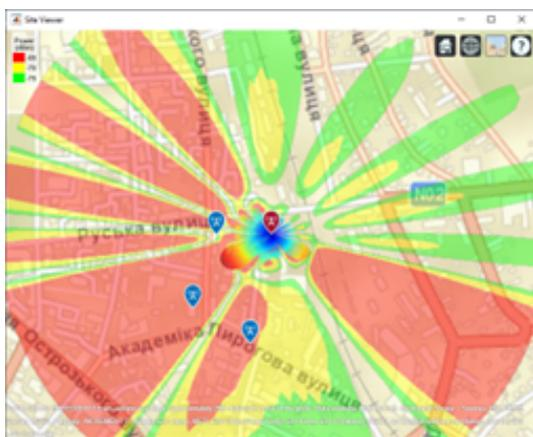
Fig. 10: Antenna beam scanning by applying a taper for an angle of -30 degrees (projection onto the terrain surface).
