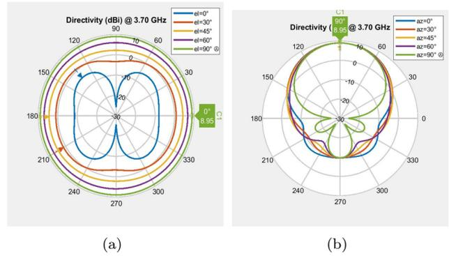
Fig. 3: An azimuth (a) and elevation (b) cut of directivity at 0, 30 45, 60 and 90 degrees elevation/azimuth.
