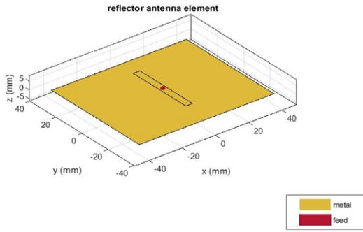
Fig. 1: Geometric dimensions of a single antenna element of the active phased array antenna.
