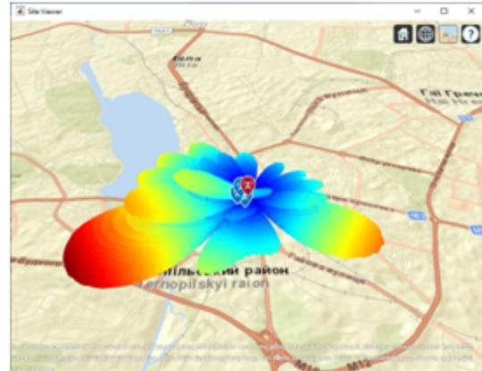
**Fig. 7:** Antenna beam scanning by applying a taper for an angle of -30 degrees in 3-dimensional coordinates.
