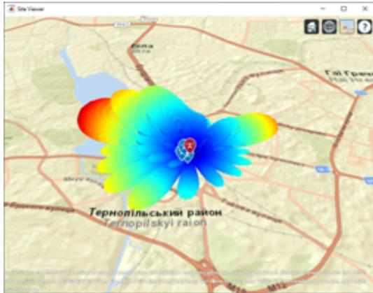
Fig. 9: Antenna beam scanning by applying a taper for an angle of +30 degrees in 3-dimensional coordinates.
