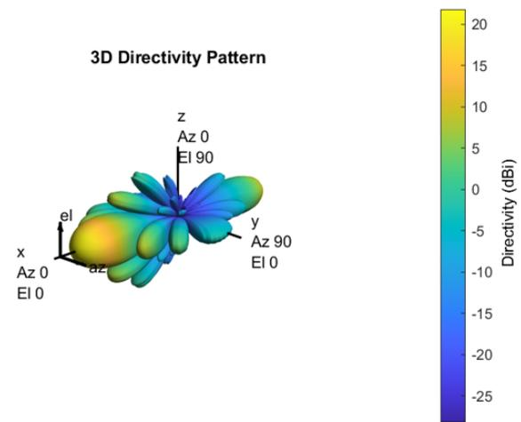
Fig. 4: Directivity diagram of a 7-by-7 phased array antenna in 3-dimensional coordinates.
