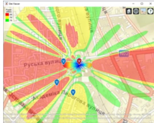
Fig. 11: Antenna beam scanning by applying a taper for an angle of 0 degrees (projection onto the terrain surface).
