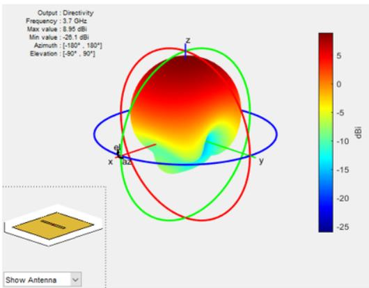
Fig. 2: Directivity diagram of a phased array antenna element plotted in 3-dimensional coordinates.
