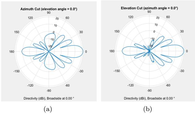
**Fig. 5:** An azimuth (a) and elevation (b) cut of directivity diagram of a 7-by-7 phased array antenna in 2-dimensional coordinates.
