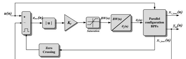
Fig. 5: Adaptive algorithm of  $\theta_2$  with proportional control of the ME
