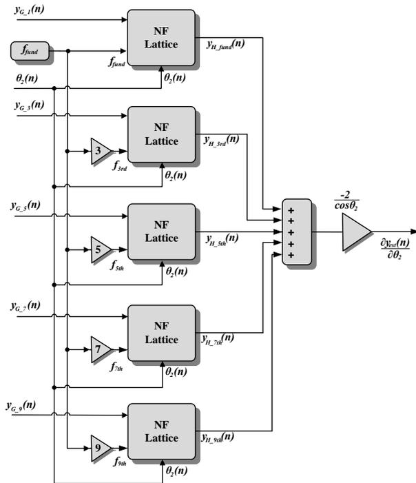
Fig. 3: Generation of the gradient of  $\theta_2$  for the parallel lattice configuration.
