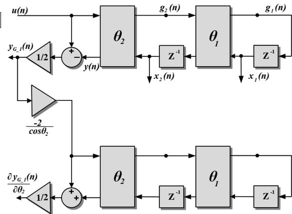
Fig. 2: Generation of the gradient of  $\theta_2$  for a single lattice filter.
