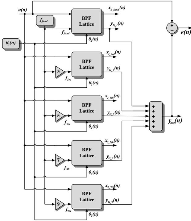
Fig. 1: Parallel configuration of second-order BPF's.
