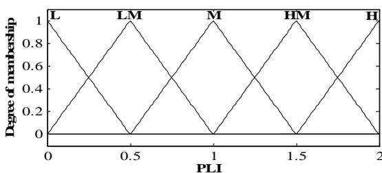
Fig. 3: Power loss indices PLI membership functions.
