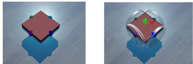
Fig. 2: Visualization in Webots of the aquatic *RoboWood* prototype (left); clicking on it, the software makes the propellers visible (right).
