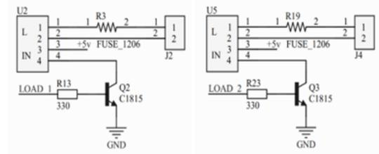
Fig. 6: Schematic diagram of the capacity block.
