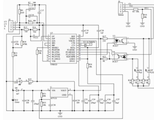
Fig. 4: Schematic diagram of solar power parameter measurement block.
