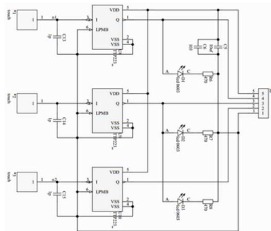
Fig. 7: Schematic diagram of touch button block.
