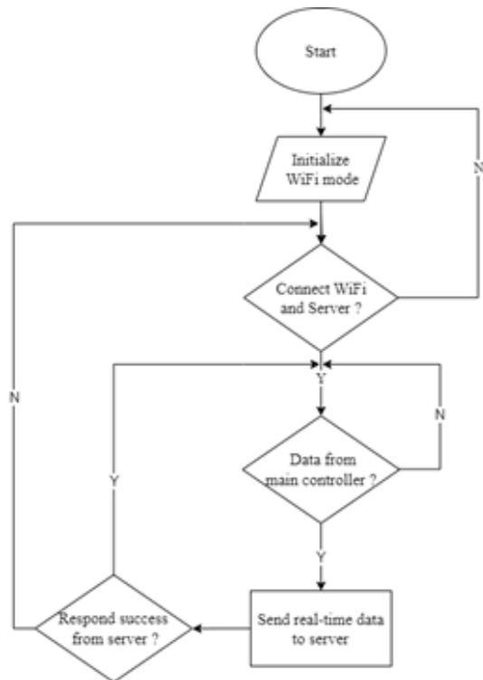
Fig. 9: Flowchart processes data and sends it to the server of the WiFi module.
