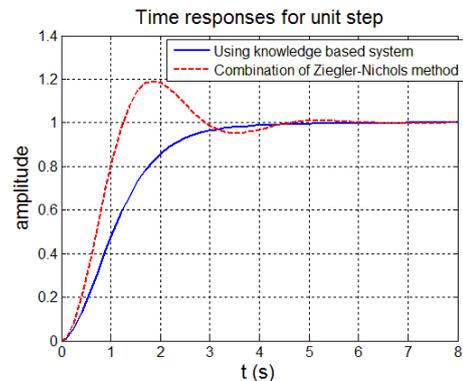
**Fig. 8:** Time response of the closed feedback loop with a PID controller with parameters determined using created the knowledge based system and a combination of classical Ziegler-Nichols methods for a unit step.
