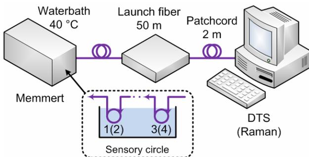
Fig. 17: The calibration of the sensory rings in option A in the water bath Memmert. The temperature of the water bath was 40  $^{\circ}\text{C}$ .
