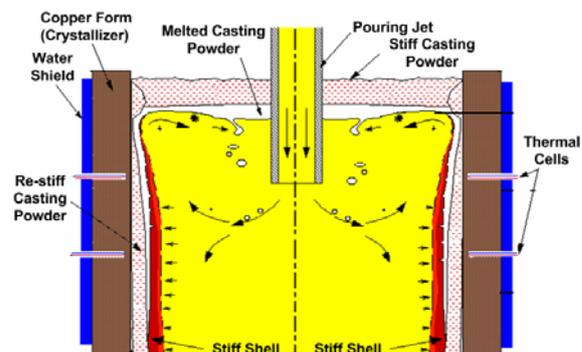
Fig. 1: The crystallizer's operation scheme [2].
