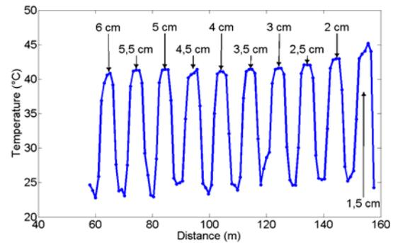
**Fig. 4:** Effect of the inner diameter of the sensory ring on the measured temperature of the water bath (measured together, optical fiber with primary protection, outer diameter 250  $\mu\text{m}$ ).
