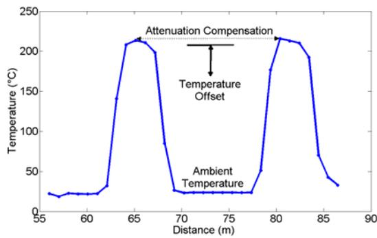
**Fig. 5:** Thermal curves of chosen configuration allowing method analysis in terms of maintaining the temperature offset calibration and compensation of the optical fiber attenuation at high temperatures.
