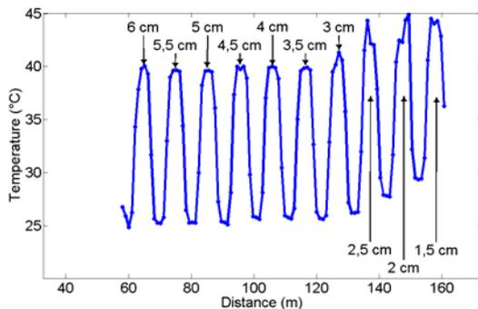
**Fig. 3:** Effect of the inner diameter of the sensory ring on the measured temperature of the water bath (measured together, optical fiber with tight secondary protection, outer diameter 900  $\mu\text{m}$ ).
