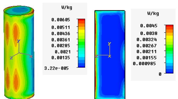
Fig. 8: Distribution of SAR (10 g) in the cylindrical model of  $h = 1,8$  m and ratio 3:1 (height: width) at 200 MHz.
