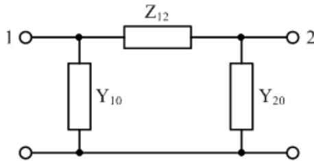
**Fig. 3:** Diagram of transmission lines.
