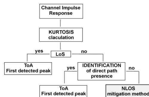
Fig. 1: Diagram of the ToA estimation for different types of communication channel.
