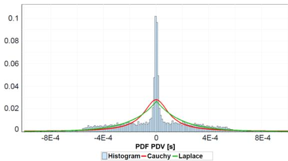
**Fig. 7:** Approximation of PDV PDF computed between the input of SW1 and output of DSLAM for two IPTV stream with the Cauchy and Laplace PDF.
