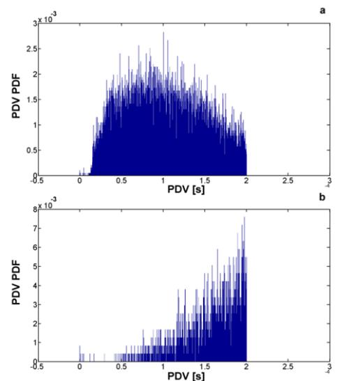
Fig. 4: PDF of RFC 3550 PDV between the nodes SW1 and DSLAM for one IPTV stream (a) and between SW1 and DSLAM for two IPTV streams (b).
