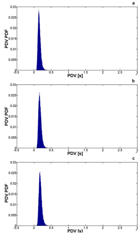
Fig. 3: PDF of RFC 3550 PDV between the nodes SW1 and SW2 (a), SW1 and SW3 (b) and SW1 and SW4 (c) for a selected IPTV stream.
