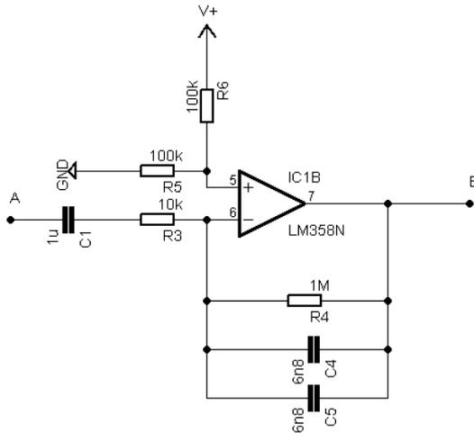
Fig. 2: First amplifier stage.
