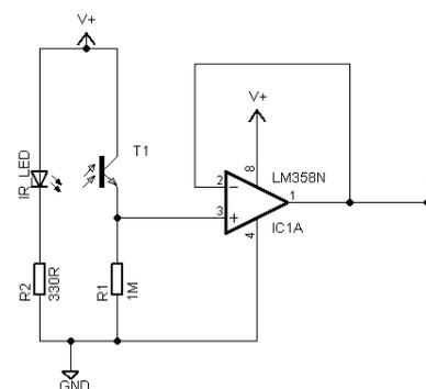
Fig. 1: Sensor circuit.
