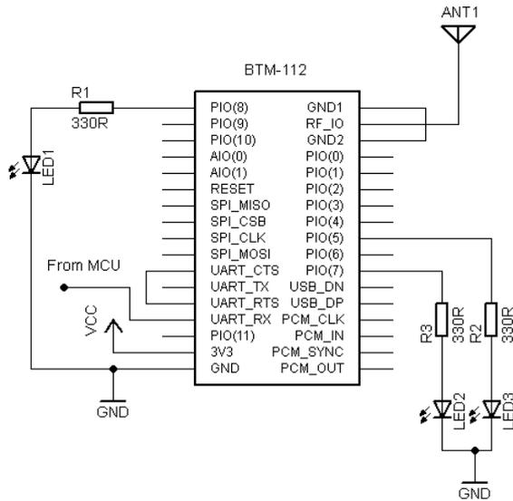
Fig. 11: BTM-112 – circuit diagram.
