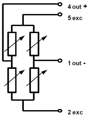
Fig. 5: Internal pressure sensor circuit (adapted from manufacturers datasheet).
