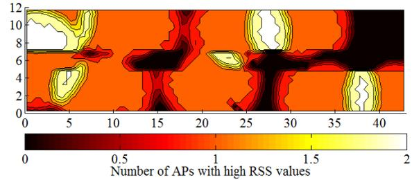
Fig. 12: Distribution of APs with RSS values higher than  $-65 \text{ dBm}$ .
