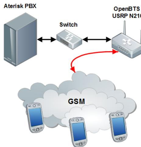
Fig. 4: Measurement schema for quality testing with components.
