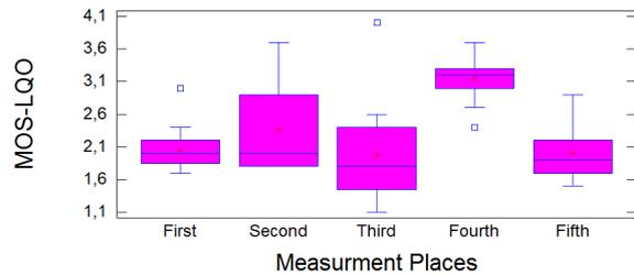
Fig. 11: PESQ method results for all measurements point. The Y axis explains mean opinion score from 1 to 5.
