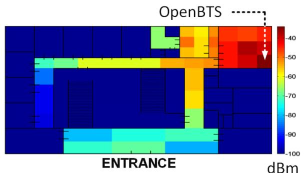
Fig. 13: Power of signal in the ground floor.
