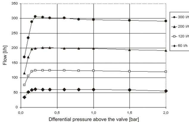
**Fig. 4:** Dependency between differential pressure above the valve and flow through the valve.
