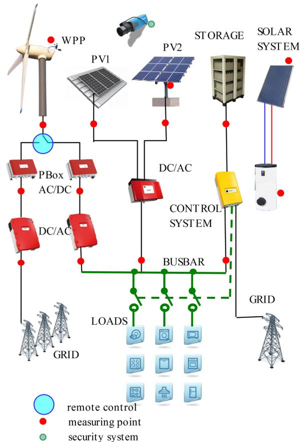
Fig. 1: The block scheme of off-grid power system.
